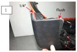
Raise and support the front of the vehicle to access the bottom of the chin spoiler. Locate the Winglet by placing it flush against the back edge of the chin spoiler and 1/4" off the bumper cover. 1/4" gap is recommended, the winglet can be moved in or out as desired.
