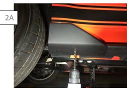
With an extra set of hands or painters tape, hold, and carefully drill (3) 1/4" mounting holes. \*\* See installation notes at the top of the page\*\* Secure the Winglet with the supplied push clips. .
