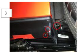
Remove the rocker panel trim piece by removing the fender liner clip and unscrewing the 2 T20 Torx screws.
