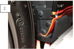
Locate the Winglet by placing it against the fender lip. Then space the Winglet 1/4" off the rocker panel. 1/4" gap is recommended, the winglet can be moved in or out as desired.
