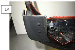
Carefully drill (4) 1/4" mounting holes. \*\* See installation notes at the top of the page\*\*. Secure the Winglet with the supplied push clips.
