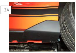
Locate the rear rocker winglet the same as steps 2-2A. \*\* See installation notes at the top of the page\*\*. Secure the Winglet with the supplied push clips.
